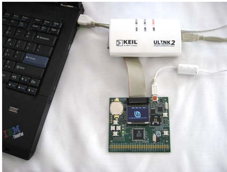
Figure 2 Hardware Connections: LM3S1968 and ULINK2
